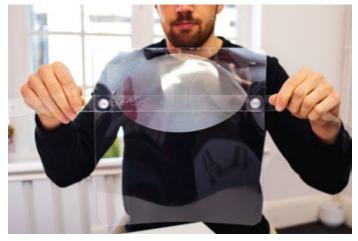
Using another plastic rivet, and the next set of 5 holes on the strap, set the head strap position on the opposite side of the face shield. The 5 holes allow you to adjust the curvature of the mask and forehead guard as desired.
